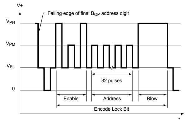
Figure 9. Pulse sequence to encode lock bit
