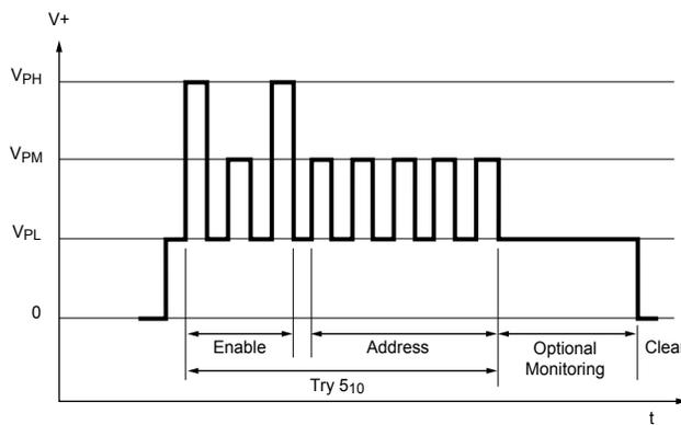
Figure 5. Pulse sequence to provisionally try calibration value 5.
